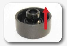
**Step 3:** Remove the lense from the focus ring by pushing the lense to the back. If the lense doesn't move please carefully heat up the ring and try again.
